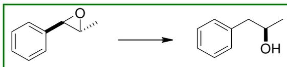
Experimental Conditions: 5 mol% Pd(0) EnCat™ 30NP, EtOAc, 4 equiv. HCOOH, 4 equiv. NEt<sub>3</sub>, 23°C, 26 hours
